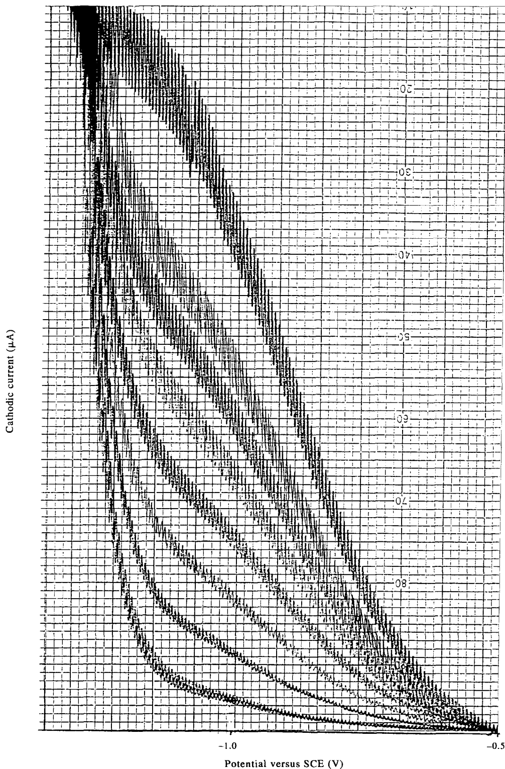
Fig. 2. Formation of \text{H}_2\text{O}_2 during the photosensitized decomposition of 2 \times 10^{-3} M ascorbic acid in the presence of 3.2 \times 10^{-5} M riboflavin at 25^\circ\text{C} . Polarograms were taken after 5 min irradiation.
